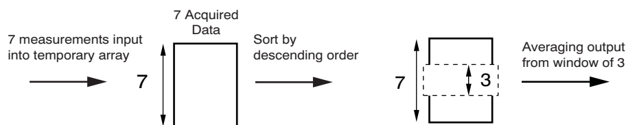
Figure 28. MAV Filter Operation (Patent Pending)
