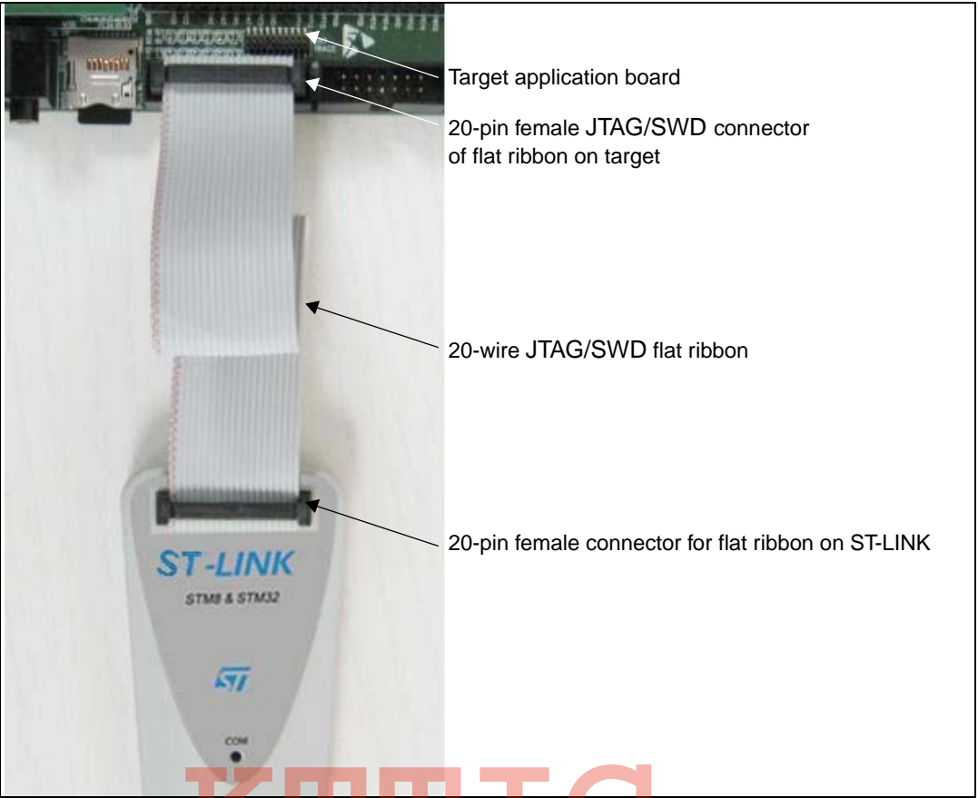
Figure 9. JTAG debugging flat ribbon layout
