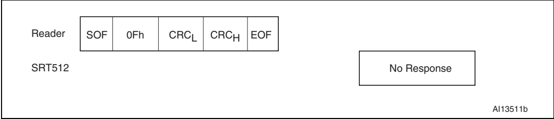
Figure 55. Completion frame exchange between reader and SRT512
