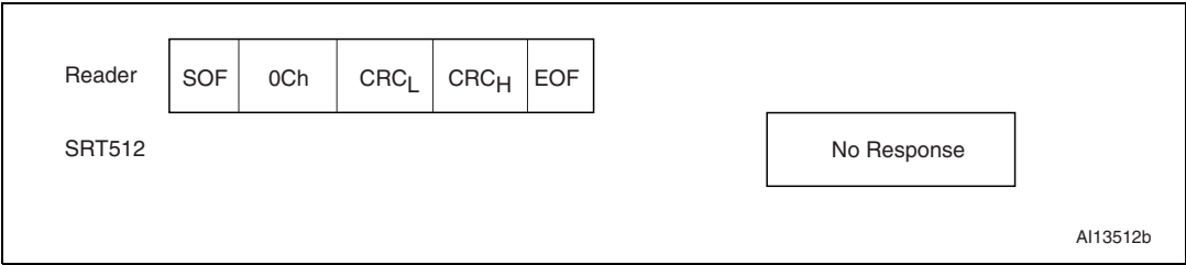
Figure 56. Reset_to_inventory frame exchange between reader and SRT512
