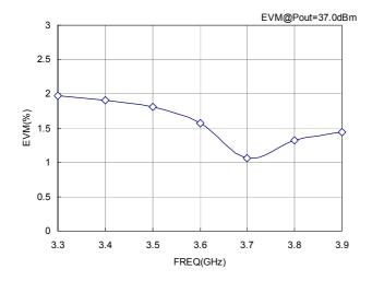
Test Condition: Vds=12V, Idq=1.5A, Pout=37dBm, Ta=25deg.C WiMAX : 64QAM-3/4,Bw=7MHz
