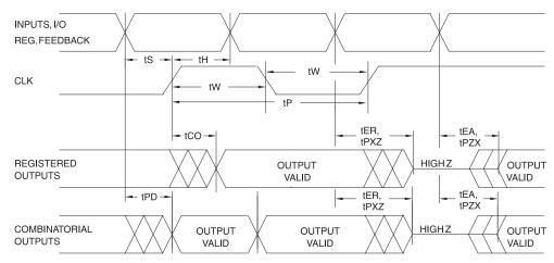
Note: Timing measurement reference is 1.5V. Input AC driving levels are 0.0V and 3.0V, unless otherwise specified. 1.
