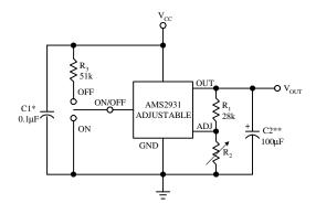
$V_{OUT} = V_{REF} \times (R_1 + R_2)/R_1$
